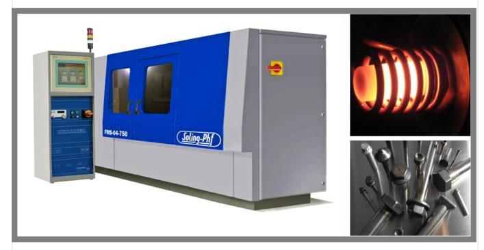
Fully AUTOMATIC HOT FORGING Machines with, Automatic Feeder and Touch Panel for easy set up and storing of product settings. All machines are easy and quick to set up and include a pyrometer for the accurate heat control, to heat and form all kinds of harden and soft steel as well as exotic alloys, such as Titanium, Inconel, Monel and Waspaloy to produce Fasteners, Ejector Pins, Punches, Cutting Tools and parts for the Automotive Industry.
